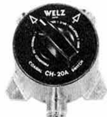
CH-20A COAX SWITCH 2kW PEP 0-900MHz 0.1 dB LOSS 60dB ISOLATION DOUBLE CAVITY £15.95
